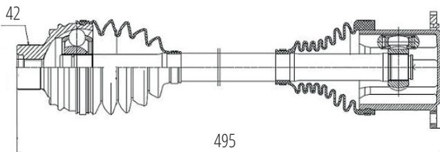
A4/A5/Q5 2.0 Tdi Tfsi (08...) (42 Roda X 495mm)
