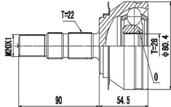
Corsa 1.0,1.4,1.6 (94/03) Celta 1.0/1.4 8V (00...06), Corsa Classic 1.0/1.6 (04...07), Novo Corsa (02...14), Prisma 1.0/1.4 (07...15), Montana 1.4 8V Eixo Gkn (10...15) (Rosca Interna Ângulo 45Graus) (22 Roda X 28 Câmbio X Trava EL) (Exceto eixo delphi) (Substitui o DG80090)
