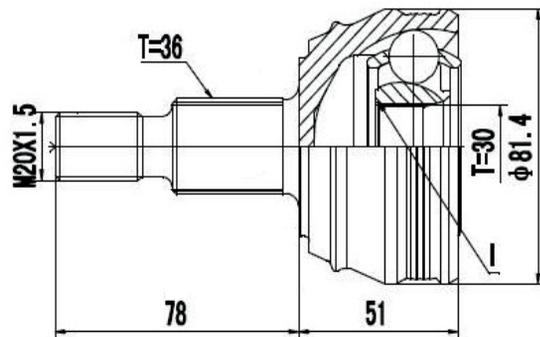
A3 1.6 (99...06), A3 1.8 (99...06), TT 1.8 20V Turbo/Turbo Quattro (99...06) (36 Roda X 30 Câmbio X Trava IL)
