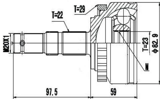
Meriva 1.8 8V/16V (03...06), Corsa Novo 1.8 8V (02...12), Montana 1.8 8V (06...) (Tds Eixo Gkn) (22 Roda X 23 Câmbio X 29 Abs X Trava ML)
