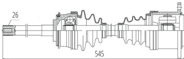
Hilux 2.8 4X4 Dana (00...06), Hilux 2.8 4X4 (92...99), Hilux 3.0 4X4 (97...05) (Completo com Tulipa) (26 Roda X 545mm)
