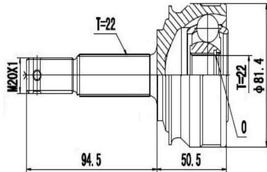
Corsa 1.0/1.4/1.6 (94...03), Corsa Pick-Up 1.6 8V (95...03), Corsa Classic 1.0 VHC/1.6 (04...13), Montana 1.8 8V (04...10) (Com Eixo Delphi) (22 Roda X 22 Câmbio X Trava EL)
