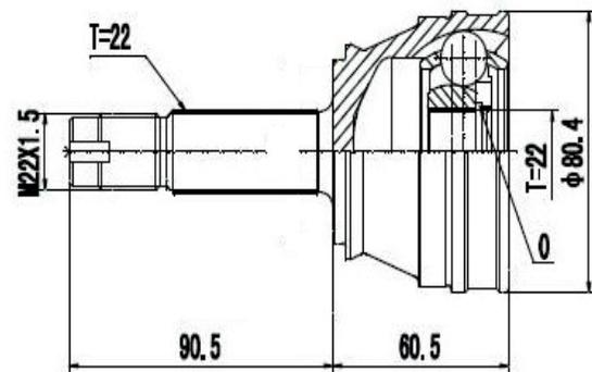
Fiorino 1.6 (96...), Palio 1.5 (96...04), Palio 1.6 8V/16V /1.7 Diesel (96...00), Palio Weekend 1.5 8V/1.6 8V/16V (97...00), Siena 1.5 8V/1.6 8V/16V / 1.7 Diesel (22 Roda X 22 Câmbio X Trava EL)
