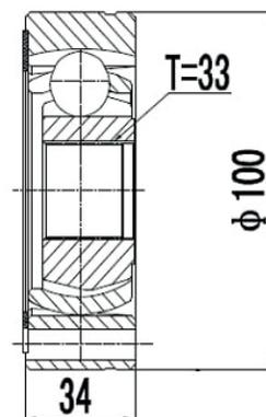
Crossfox Flex 1.6 8V (05...08), Fox Flex 1.6 8V (07), Polo Hatch 1.6/2.0 (03...07), Spacefox Flex 1.6 8V (07...), Gol 1.6 8V (09...13), Gol 1.0 Turbo (00...06), Parati 1.0 Turbo (00...06) (33 Estrias)
