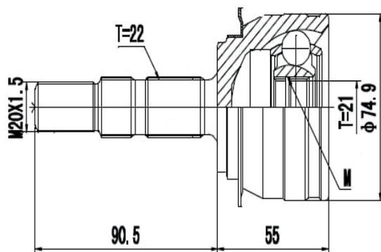
Agile 1.4 (09...), Montana 1.4 (11...), Celta 1.0 (13...15), Corsa Hatch 1.0 (09...10), Corsa Hatch 1.4 (13...15) (22 Roda X 21 Câmbio X Trava ML)
