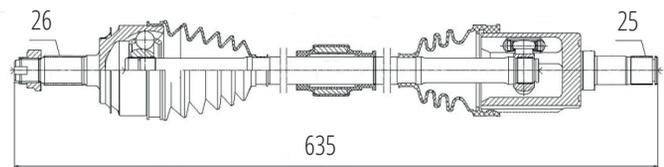
Esquerdo Manual/Automático New Fit 1.4 (09...14), New Fit 1.5 (09...14), City 1.5 (09...14) (26 Roda X 25 Câmbio X 635mm)
