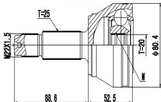
Fiesta 1.0 Zetec Rocam (99...06), Ka 1.0 Zetec Rocam (00...14) (25 Roda X 20 Câmbio X Trava ML)
