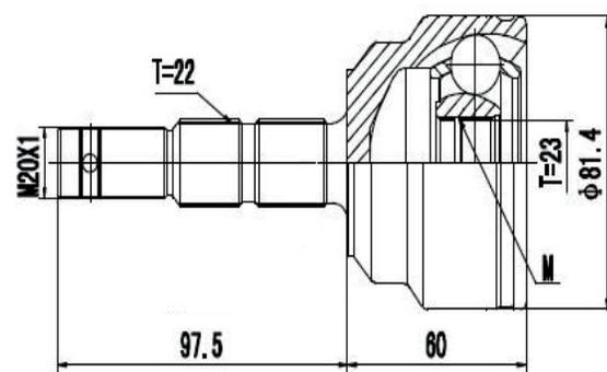
Corsa 1.6 (94...03), Corsa Novo 1.8 8V (02...12), Meriva 1.4 8V (06...), Meriva 1.8 8V/16V (03...06), Montana 1.8 8V (04...) (22 Roda X 23 Câmbio X Trava ML)
