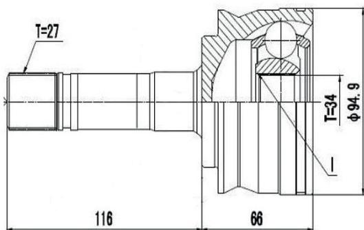
Ranger 2.5 4X4 Turbo Diesel (98...00) (Sem Roda Livre) (27 Roda X 34 Câmbio X Trava IL)
