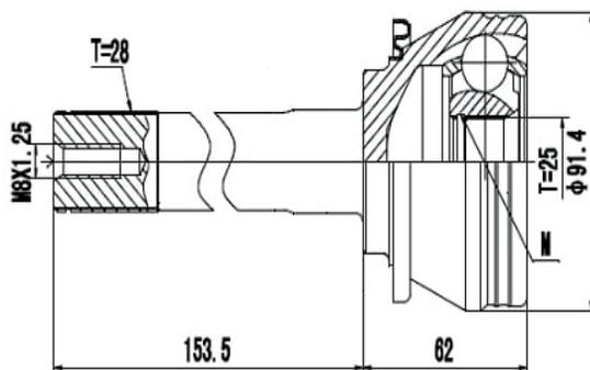
L200 2.5 4X4 (98...04), L200 Outdoor 2.5 HPE Diesel (03...), L200 Sport GL/GLS HPE (03...), Pajero 2.5 HPE Diesel (03...), Savana 2.5 HPE Diesel (03...) (28 Roda X 25 Câmbio X Trava ML)
