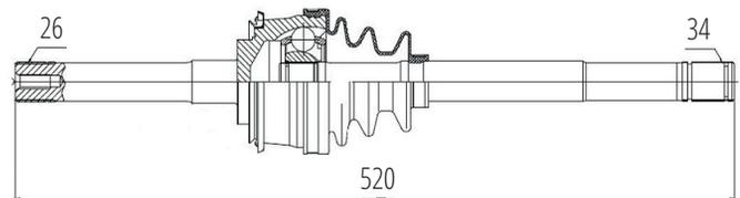
Hilux 2.8 4X4 Sohc Eixo Dana (97...08) (26 Roda X 34 Câmbio X 520mm)
