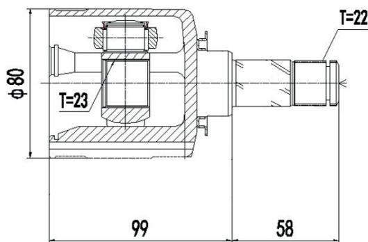
Onix 1.4 (12...), Spin 1.8 (13...), Prisma 1.4 (13...16), Novo Prisma 1.4 (12...) (22 Câmbio X 23 Trizeta X 157mm)
